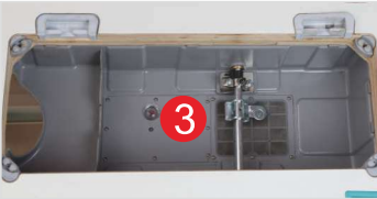
3. Sirkülayonlu yağ depolama karteri Circulating oil storage pan
