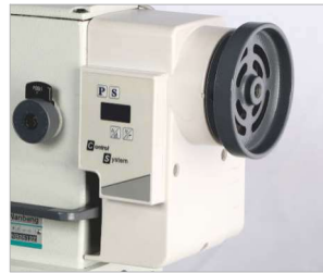
Kararlı performansa sahip 750W yüksek güçlü servo motor 750W high-power servo motor with stable performance
